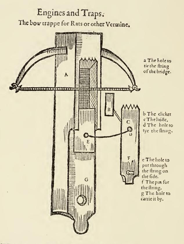
This engine of trappe with the bow, is made like a bore, of a whole piece of wood, with the lidde opening a thutting aboue, and this fide is unbent, the wing the left fide and the lidde, and this fide is unbent, the wing the left fide and the lidde, and this fide is unbent. With holes and the firing for to fet him, as more plainly thall be the wed bent and fet.
