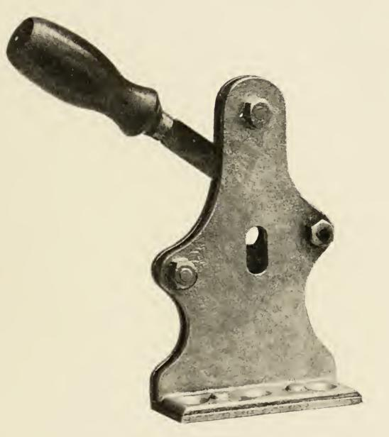
APPARATUS USED IN THE DANISH COLLECTING DEPÔTS FOR CUTTING OFF RAT-TAILS
