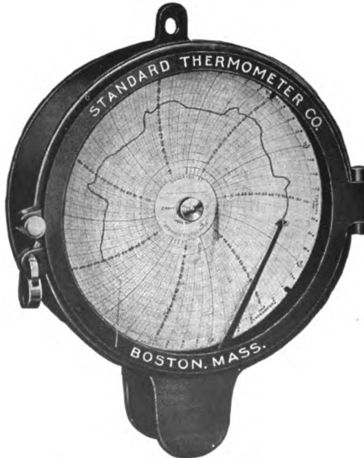
FORM OF RECORDING THERMOMETER USEFUL IN TEST OF VENTILATION
