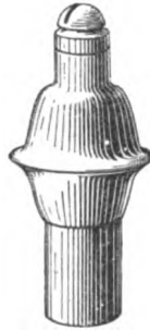
Fig. 106. Bat's-Wing or Slit Burner.
