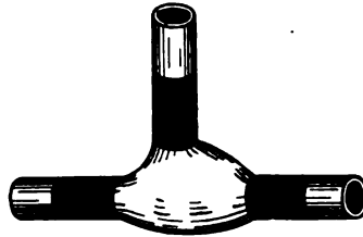
Fig. 243. Combination Branch and Round Joint.
