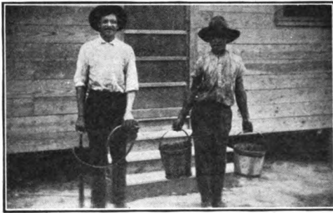
FIG. 81.—Hand-and-foot spray pump for use in applying bone black and crude oil mixture in latrines. Bone or lamp black may be of any quality provided it is fine as flour. The mixture is strained before use by passing through a sieve made of several layers of metal mosquito netting. Several spray tips should be on hand in reserve.
