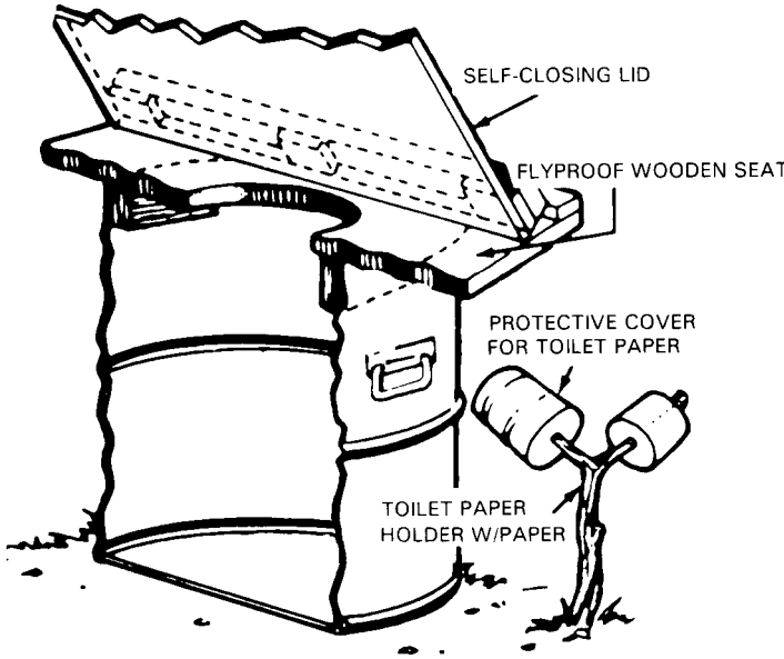
Figure B-13. Burn-out latrine.
