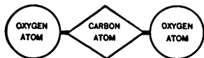
FIG. 45. A molecule of carbon dioxide. This gas is a compound, its molecules having in them two kinds of atoms.
