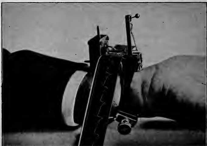
THE SPHYGMOGRAPH ON A WRIST, AND THE RECORD IT IS MAKING
