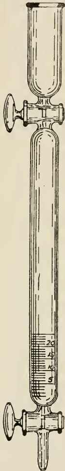
FIG. 69.—Glass Burette for Testing Percentage of Sulphur Dioxide.
