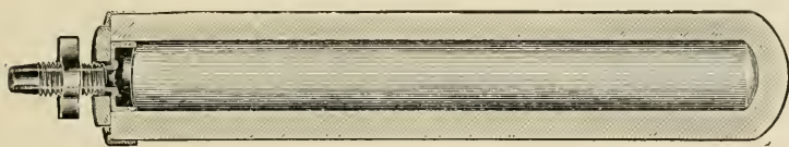
FIG. 85.—Section of 'Berkfeld' Filter Tube.
