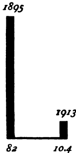
FIG. 41. In 1895 Chicago ran its sewage into Lake Michigan, from which its water supply was obtained. A drainage canal now carries most of the sewage away from the lake. The diagram shows the decrease in the death rate from typhoid fever following the improvement of the water supply.
