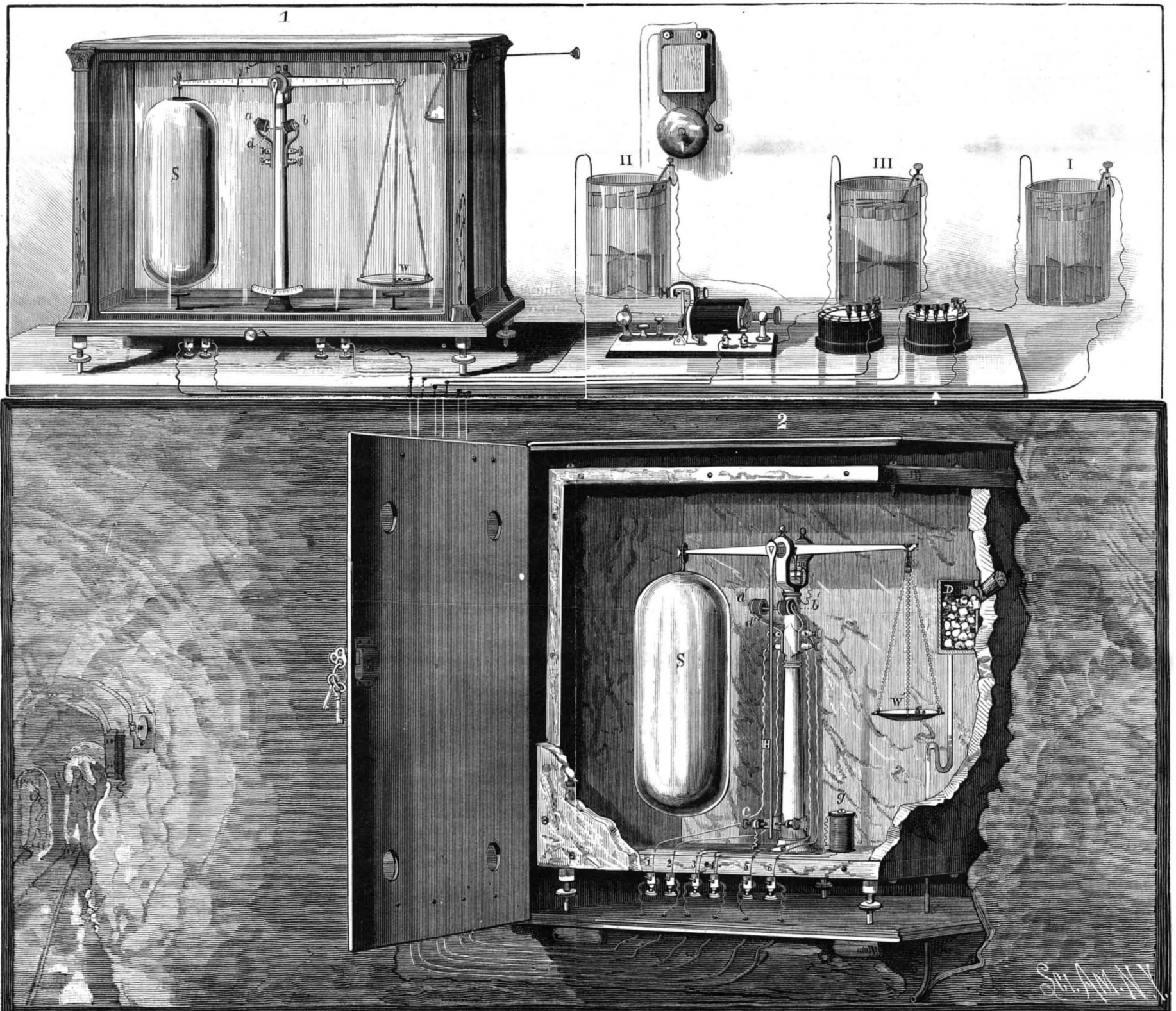
HENRY GUY CARLETON'S INSTRUMENT FOR INDICATING FIRE DAMP IN MINES.
