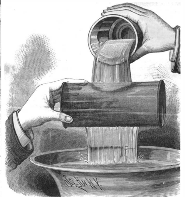
Fig. 4.—POURING WATER THROUGH FULL CYLINDER.
