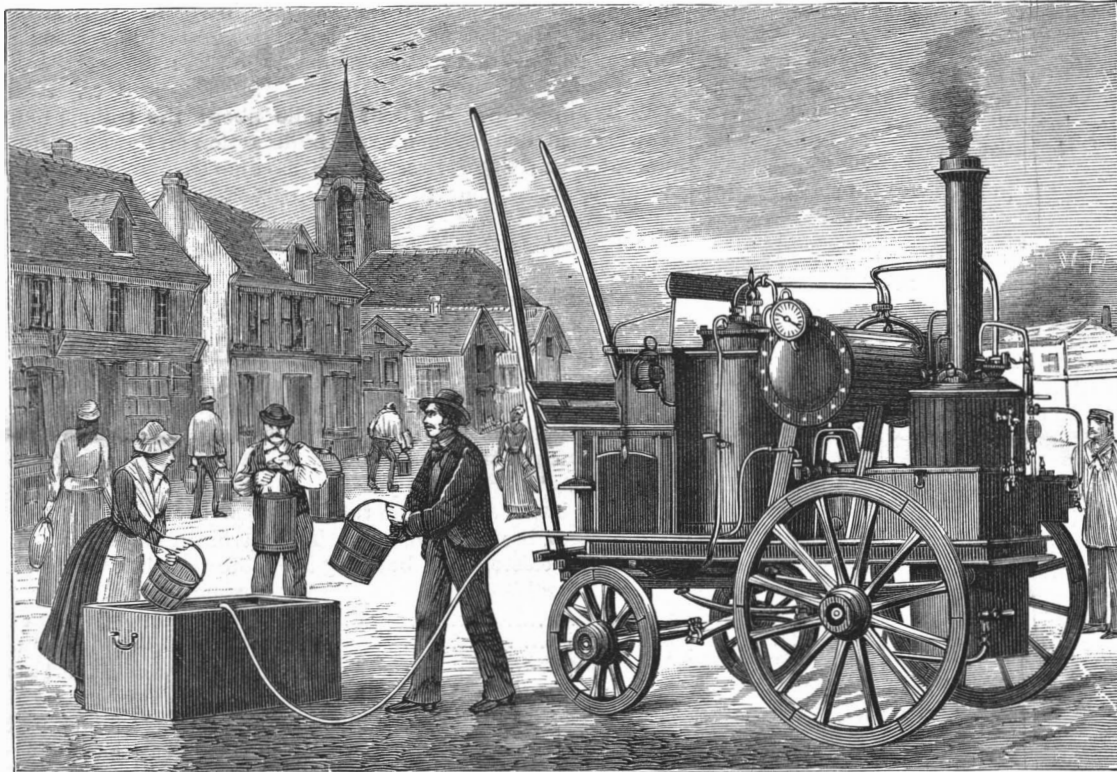
Fig. 1.—APPARATUS FOR STERILIZING WATER BY HEAT.
