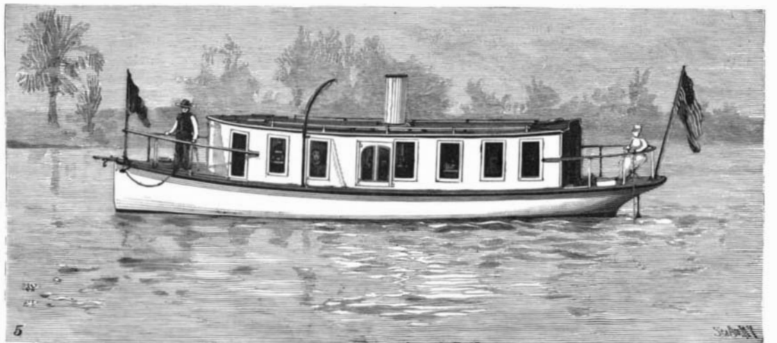
Launch 42x9 ft., with 25 I. H. P. "Union" Engine, Property of A. N. Stanton, Bridgeport, Conn.
