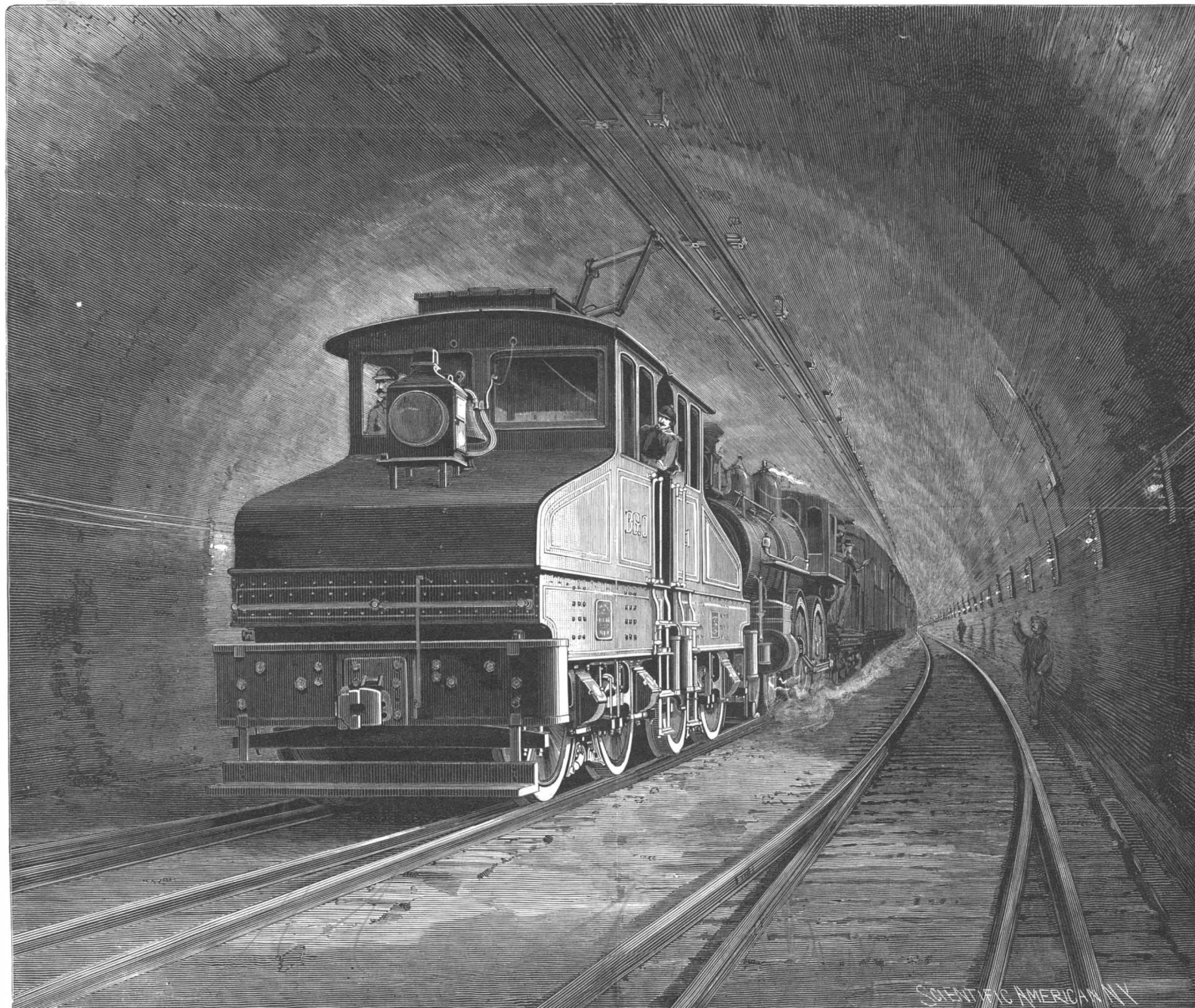
THE NEW ELECTRIC LOCOMOTIVE OF THE BALTIMORE AND OHIO RAILROAD COMPANY.—[See page 87.]
