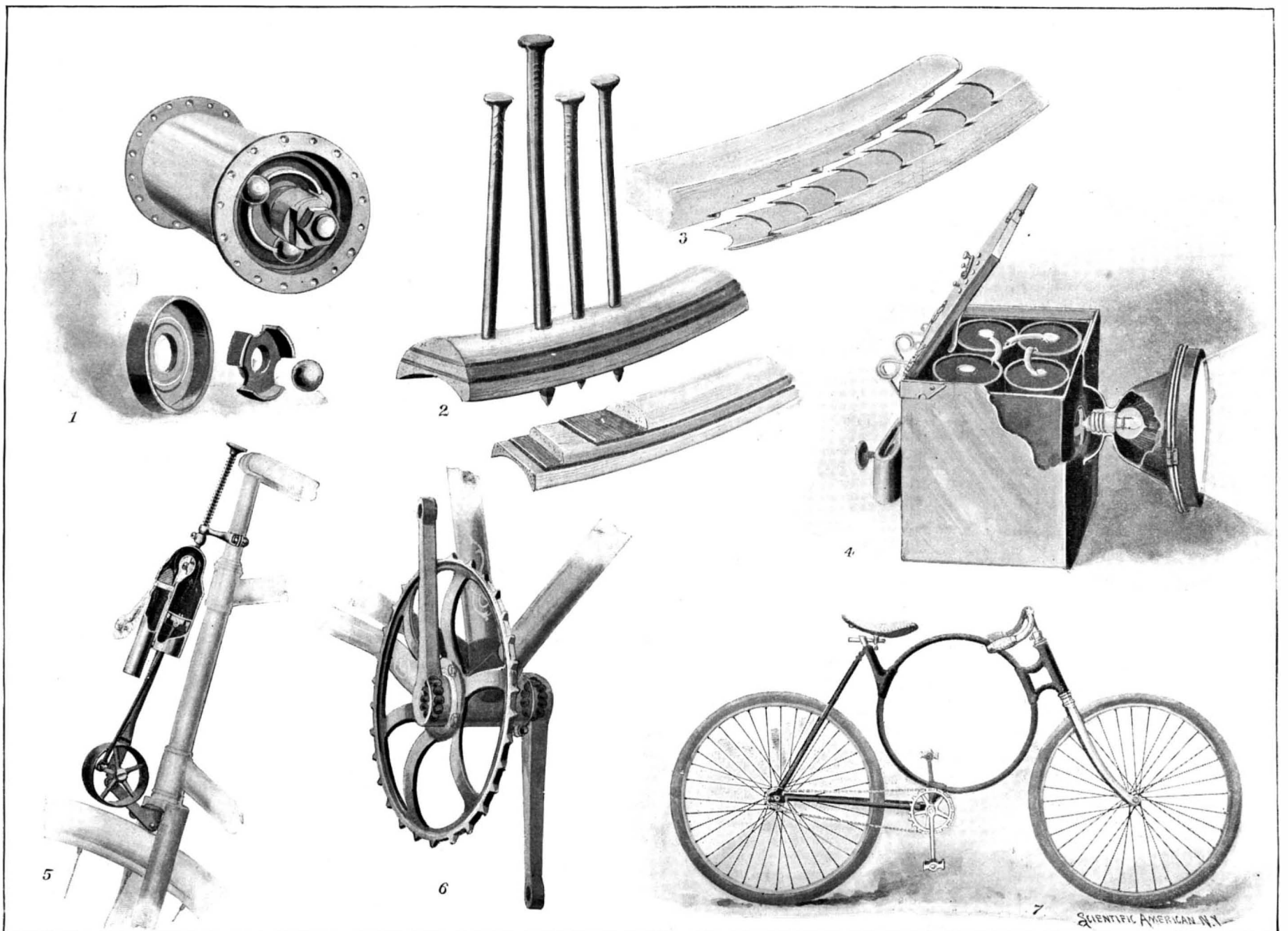
1. Three-ball bearing. 2. Non-splitable rim. 3. Joint for non-splitable rim. 4. Electric bicycle lamp. 5. Automatic whistle. 6. A device to reduce friction. 7. The circle cycle.
