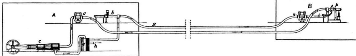
8.—DIAGRAM OF TWO-STATION ONE-COMPRESSOR LINE.
