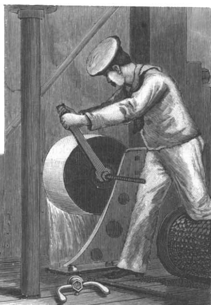
4.—Using the Wrench in Close Quarters.
