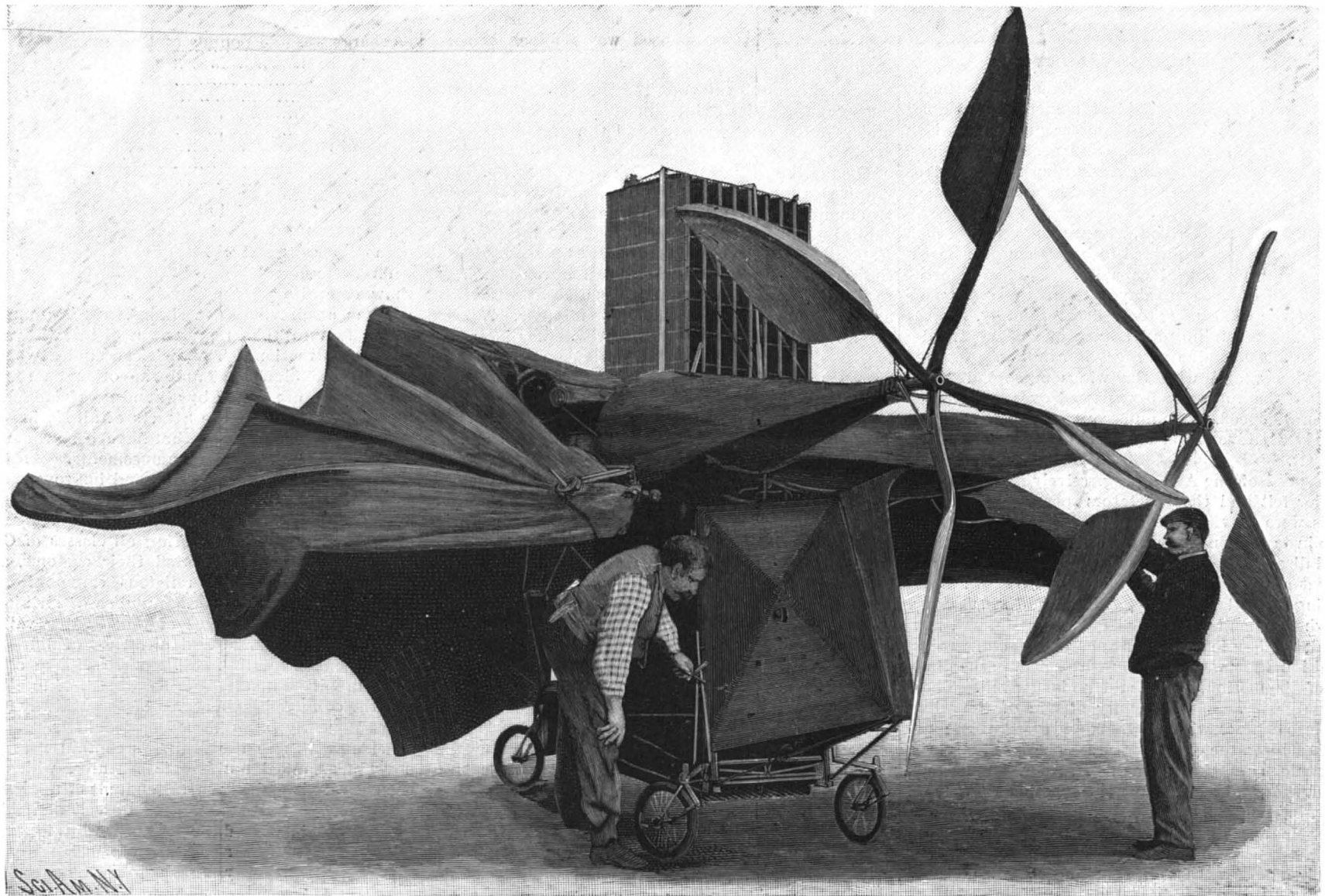
THE "AVION" WITH THE WINGS FOLDED.
