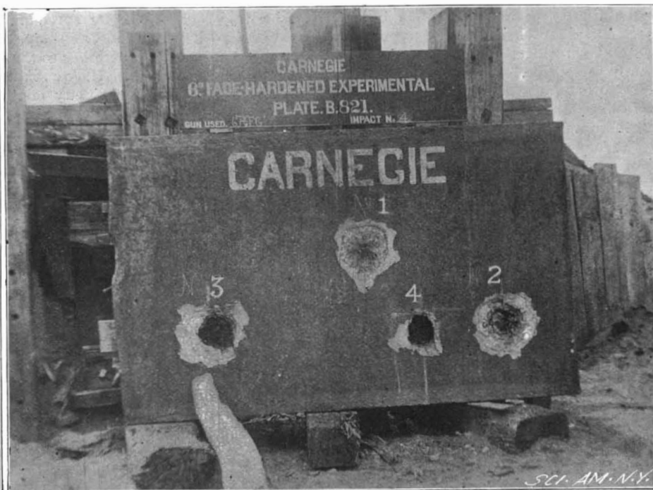
3.—SAME PLATE PENETRATED BY CAPPED SHELL DELIVERED WITH 1984 FOOT-SECONDS VELOCITY.
