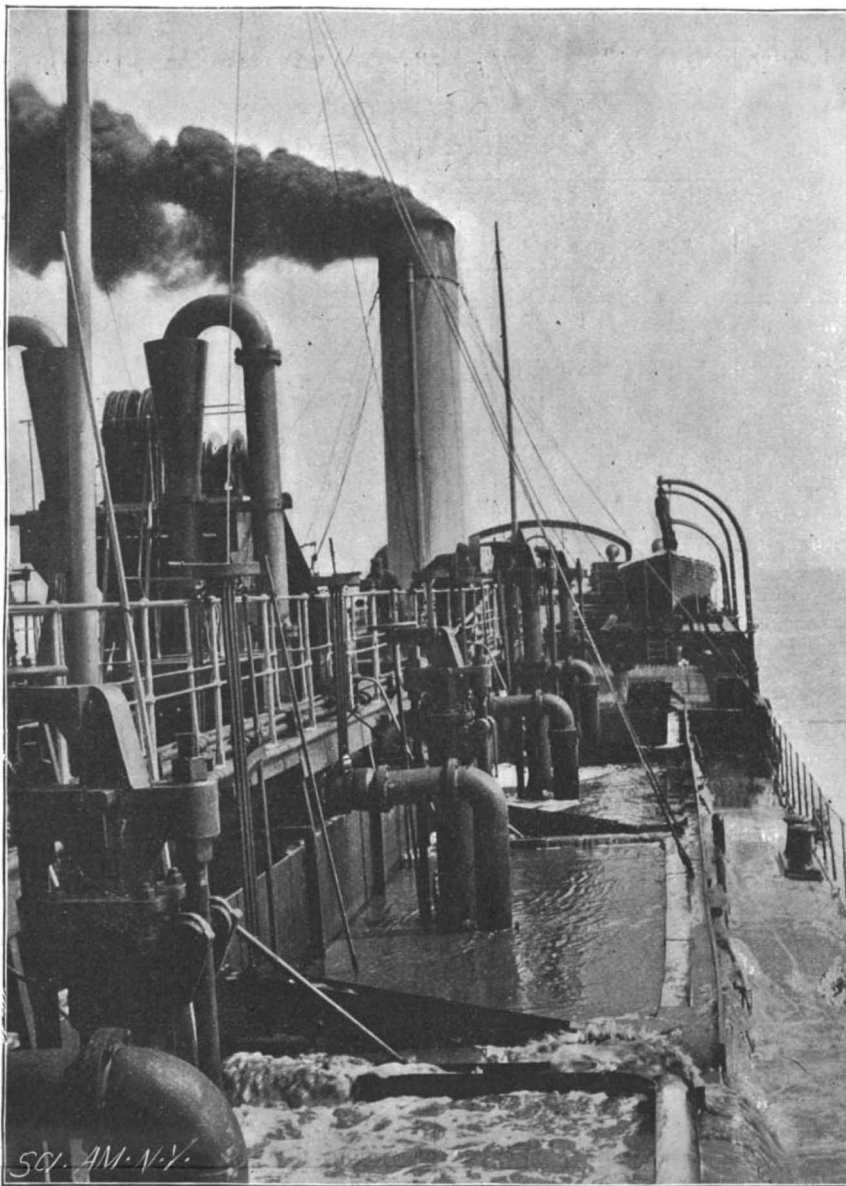
Fig. 1.—DECK VIEW OF THE "BRANCKER," SHOWING THE TANKS AND THE HYDRAULIC HOISTS FOR TANK CYLINDERS.
