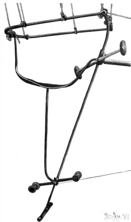
OPERATOR'S SEAT AND PROPELLING MECHANISM.
