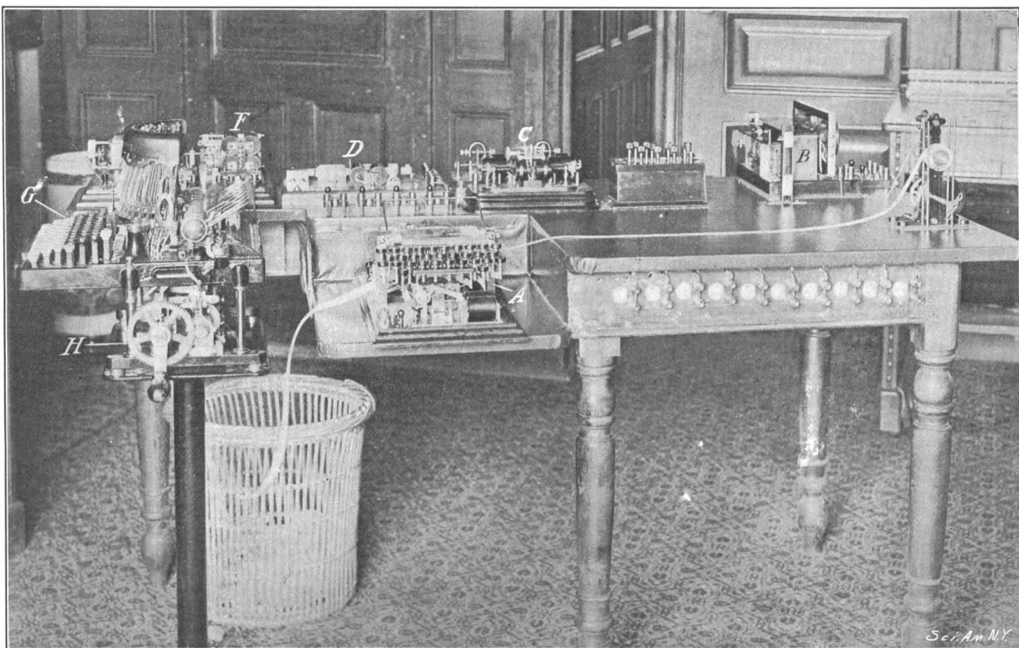
At the transmitting station the blank tape is punched with perforated characters in typewriter punching machine, A; then run through a modified Wheatstone transmitter, B. At the receiving station the impulses are controlled by relays, C, and a vibrator, D, and operate a punching magnet, F, which reproduces the perforated characters upon a blank tape. This tape is then run through an attachment, H, to a typewriter, G, which latter prints the message in page form in the Roman characters.
