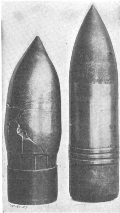
A 6-Pounder Armor-piercing Shell, Filled with Maximite Before and After Firing Through a 3-Inch Armorplate. The Shell Upset and Rebounded Without Exploding.
