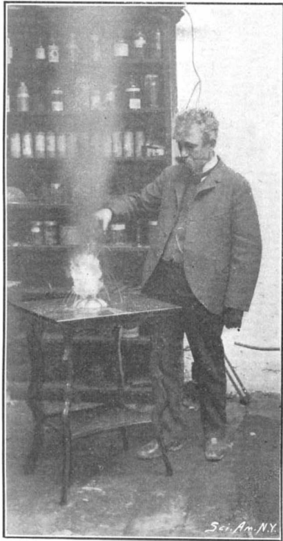
The Inventor Pouring Molten Iron Upon Maximite.
