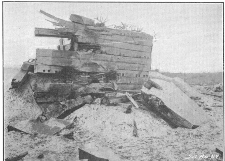
Wreck of 12-inch Plate After Penetration and Explosion of 12-inch Shell.
