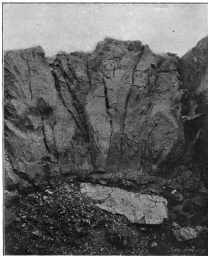
Partly Coked Contents of a Coke Oven.
