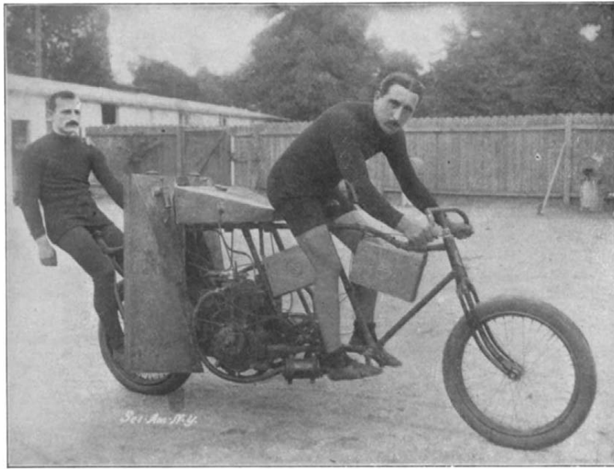
A French Motor Tandem for Pacing. (Combination Gasoline Tank and Wind Shields.)
