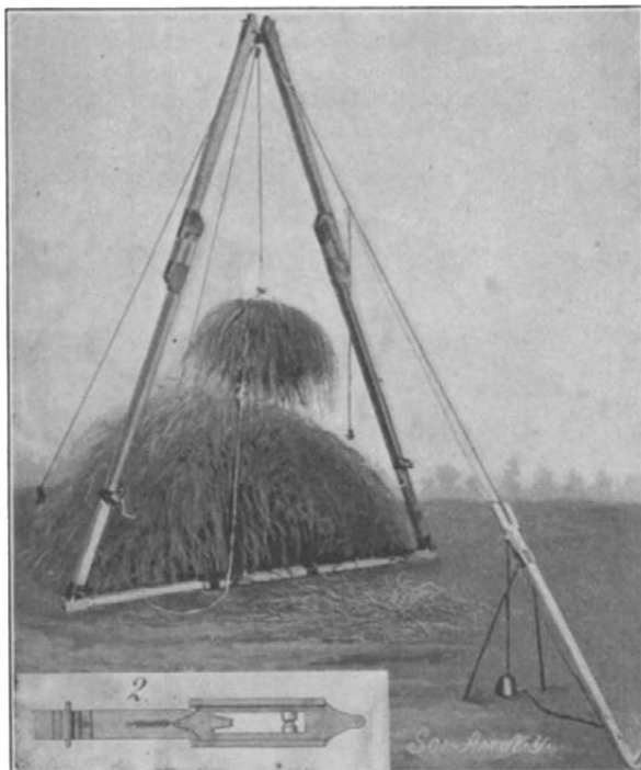
IMPROVED HAY STACKER AND BUILDERS' DERRICK.
