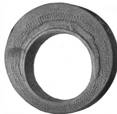
Fig. 7.—Non Puncturable Tire with Layer of Fiber.
