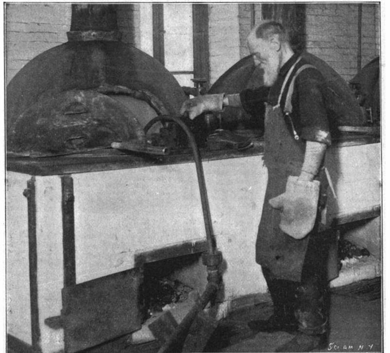
Separating the Gold from the Silver by Boiling with Sulphuric Acid.
