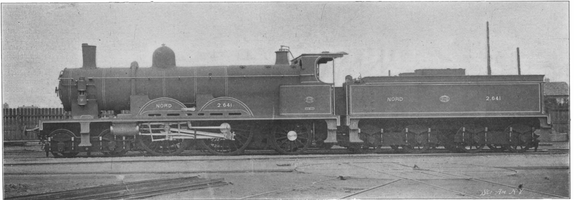
TYPE OF NEW FOUR-CYLINDER COMPOUND EXPRESS ENGINE BUILDING FOR THE GREAT WESTERN RAILWAY, ENGLAND.
