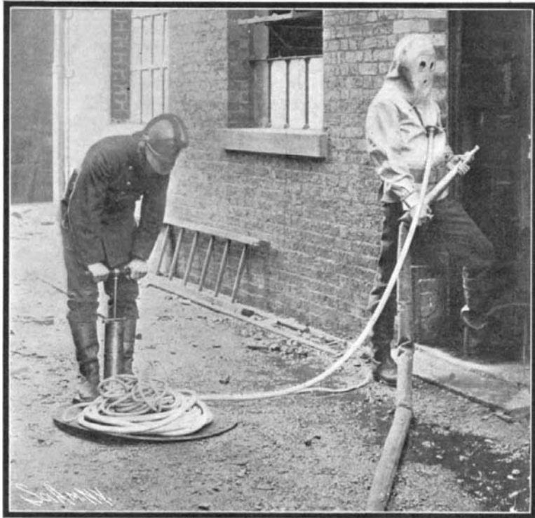
A FIREMAN CLAD IN A PROTECTIVE SUIT, TO WHICH AIR IS SUPPLIED.
