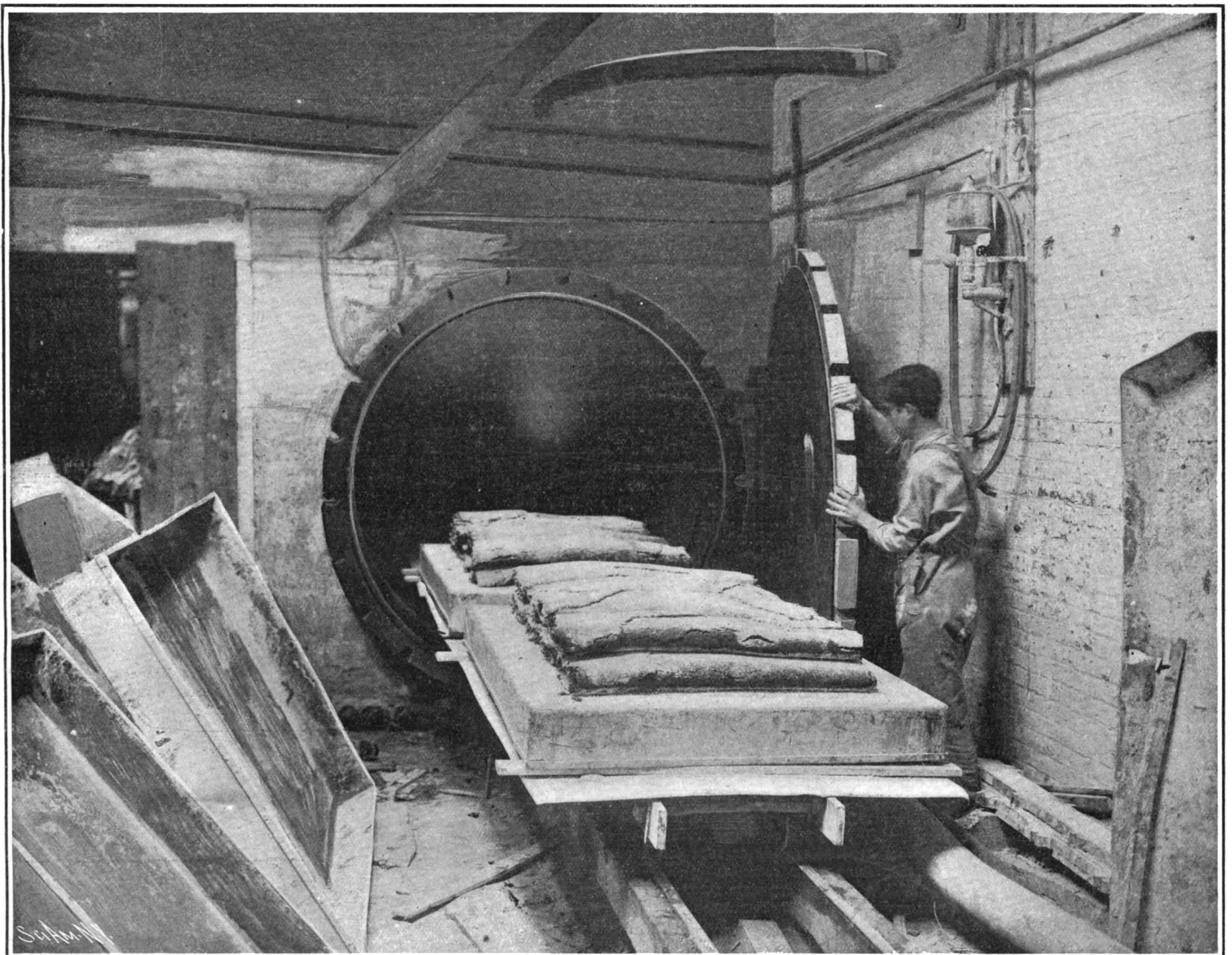
Running a Load of "Rubber Shoddy" Into the Devulcanizing Cylinder Where, Under Action of Steam Heat, the Sulphur is Extracted.
