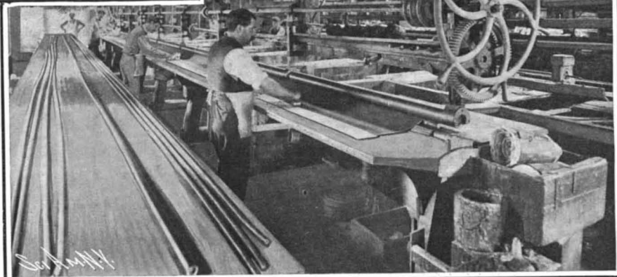
The Hose Room. Applying the Canvas Strip and Rubber Cover to the Rubber Tube.
