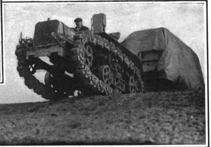
The Tractor About to Descend a Sand Bank with a 5-Ton Trailer.
