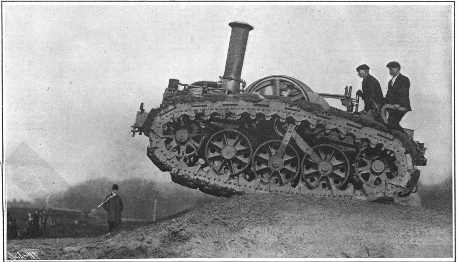
The Caterpillar Motor, Showing the Weight-Carrying wheels.
