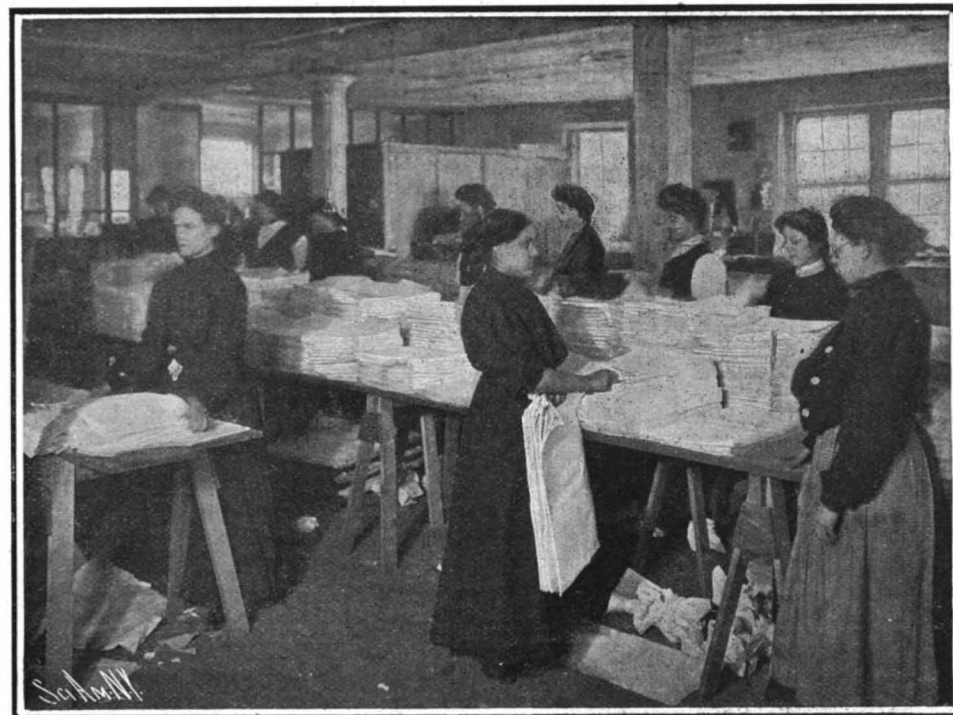
The Magazine is Assembled by Picking up a Sheet from Each Pile.
