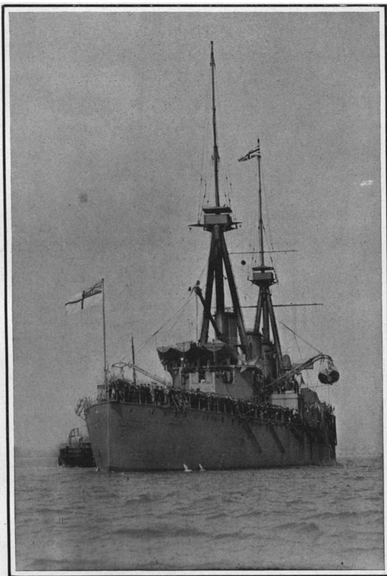
The square structure below boat davits is a temporary tank for measuring water on trial trip.
