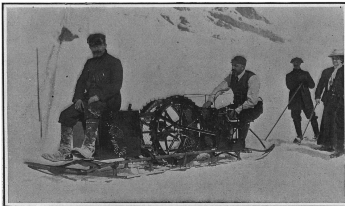
DR. CHARCOT'S MOTOR-DRIVEN SLED FOR ARCTIC EXPLORATION.
