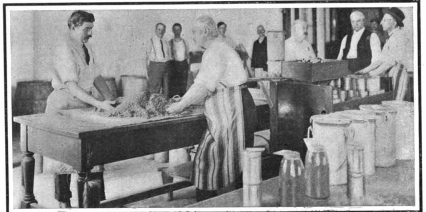
Mixing Room. Samples Received from Docks Are Thoroughly Mixed and Small Samples for the Laboratory are Prepared.
