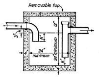
SECTION FIGURE 11.—Typical grease trap.
