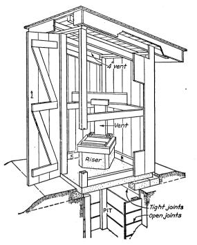
FIGURE 14.—Sanitary type of privy. Detailed plans and a bill of materials for this design can be had from the United States Public Health Service, Washington 25, D. C.
