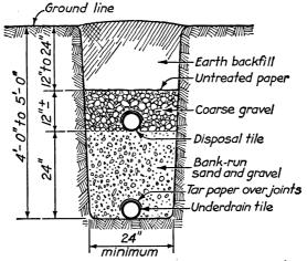
Slope of disposal tile 2 to 4 inches per 100 feet. Slope of underdrain tile not less than above. Plug upper end of underdrain-tile lines, lower end to discharge into rock-filled seepage pit or into other approved outlet.
