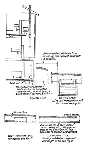
FIGURE 1.-A septic-tank system.
