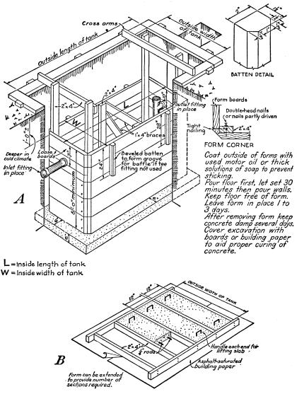
FIGURE 7.—Inside form hung in place for single-chamber septic tank, also a form for casting concrete-slab cover in sections.
