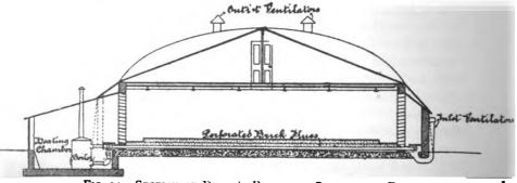
FIG. 25.—SECTION OF DUCAT'S BACTERIAL SELF-ACTING FILTER.
