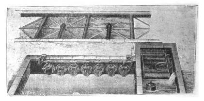
FIG. 45. RIDGWAY'S AUTOMATIC DISTRIBUTOR FOR CONTACT BEDS.
