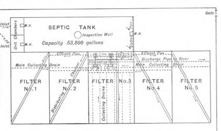
Fig. 35.—Plan of Belle Isle Sewage Works, Exeter
