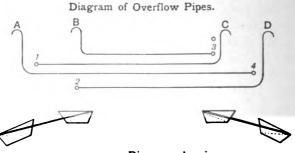
Diagram showing successive states of Filters corresponding to successive positions of alternating gear-
