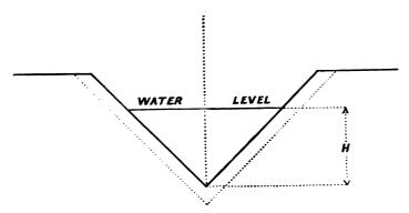
in a V notch is as the square of the height from the vertex, and the volume discharged as the ! power of that height. The formula is
