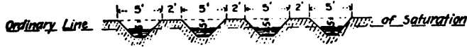
FIG. 27.—METHOD OF ADAPTING INTERMITTENT FILTRATION AREA TO CULTIVATION, BY MEANS OF ABSORPTION DITCHES.
