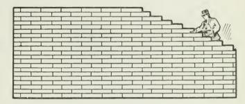
A Day's Work in Bricklaying—City Day Labor, 240 Bricks an Hour; Metropolitan Water-Board Contract, 570 Bricks an Hour.
