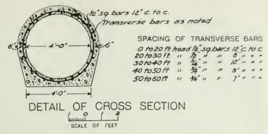
REINFORCED CONCRETE PIPE UNDER PRESSURE.
