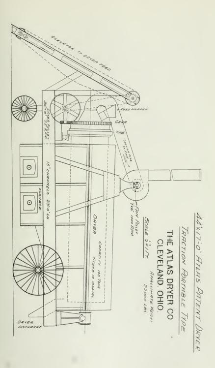
The body is of No. 10 steel plates with angle iron reinforcing frame and ends reinforced with ½ by 3-inch bars, all securely riveted and forming a practically water-tight joint between the two quadrants when closed. The panel plates securing the quadrants in position are bracketed to the axle and braced to the frame. Rollers eliminate friction on pivots and bolts supporting the body.
