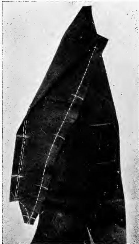
Diagram 5—Basting Underarm Seam from “Second Notch” up to the Armhole, as described in Section III.
