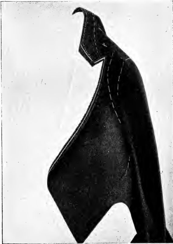
Diagram 22—Showing how a dress coat is pressed before putting on silk facing.
