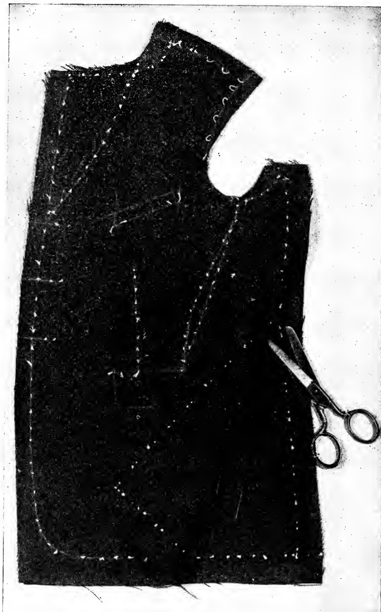
Diagram 3—Showing the Method of Putting in Marking-Stitches as described in Section II.
