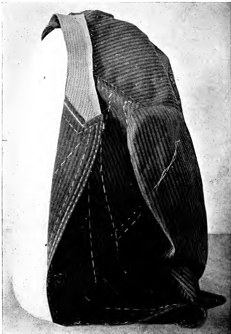
Diagram 19—This illustrates how the stripes should run straight in the back, and how the collar is prepared for shaping.
