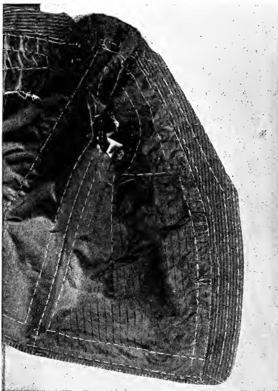
Diagram 16—Shows forepart with edge creased and placed on table, also the manner of basting as described in Section XLI.
