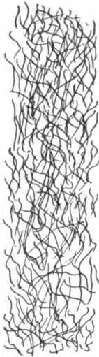
CONSTRUCTION OF WOOLEN YARNS
