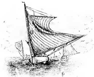
PEAK LOWERED TO AVOID "GOOSE-WING"
