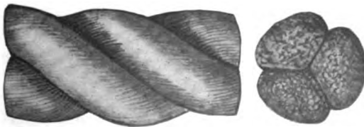
FIG. 4. CROSS SECTION, 3-STRAND ROPE.
