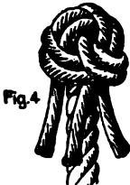
Double Wall and Double Crown or "Man Rope Knot."
