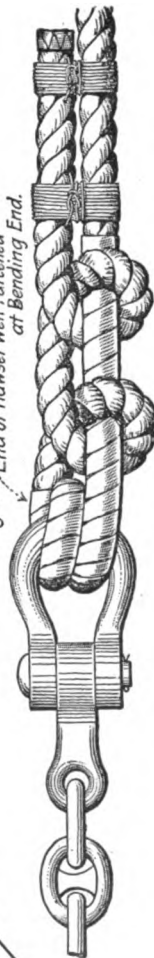
Towing a Vessel with a Manilla Hawser Bent to Bower Cable. (Anchor Shackle)
