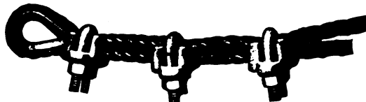
Wrong Way (U-bolt on Tension End). WIRE ROPE CLIPS,
