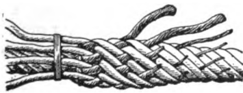
Fig. 1 A Short Splice in Wire
