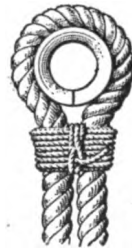
Fig. 5 Round Seizing Crossed Clove Hitch Finish
