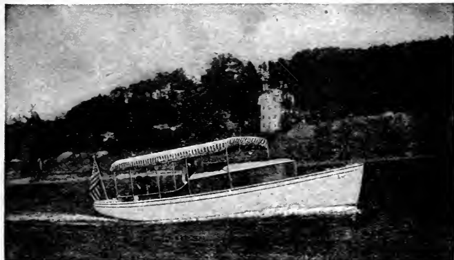
28' 8-10 H. P. Hunting Cabin Launch—Gas Engine & Power Co. and Charles L. Seabury & Co. (Consolidated.)
