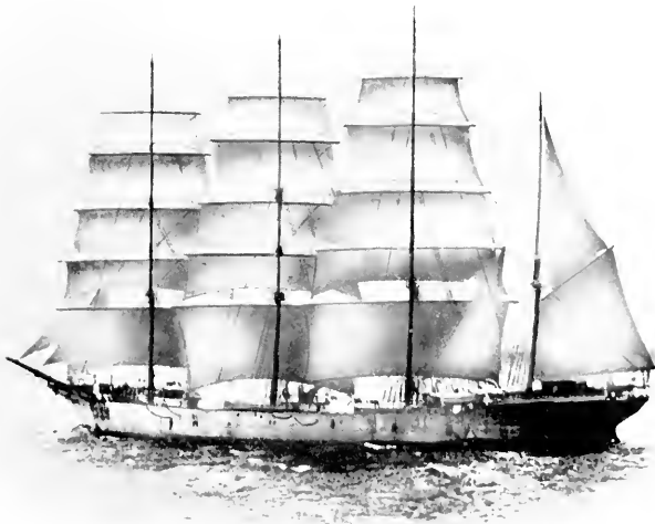
FIG. 79. THE "QUEEN MARGARET." STEEL FOUR-MASTED BARQUE. REGISTERED TONNAGE, 2144. BUILT IN 1893.
