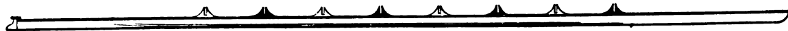
EIGHT-OARED CUTTER, 60 Feet Long. The Old Style of Racing Boat, or for Water for which the Outrigger is considered of too slight a Build.
