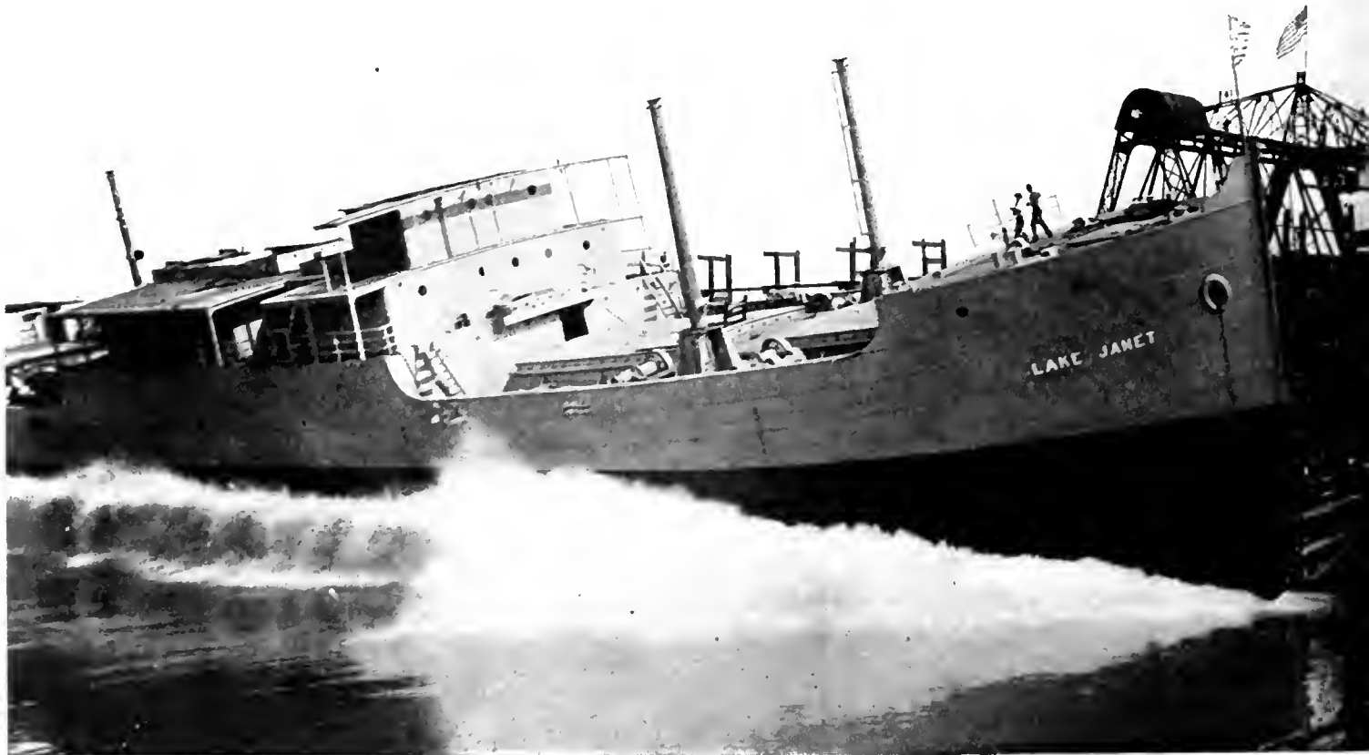
Fig. 70. A Broadside Launching at the Ecorse Yard, Great Lakes
