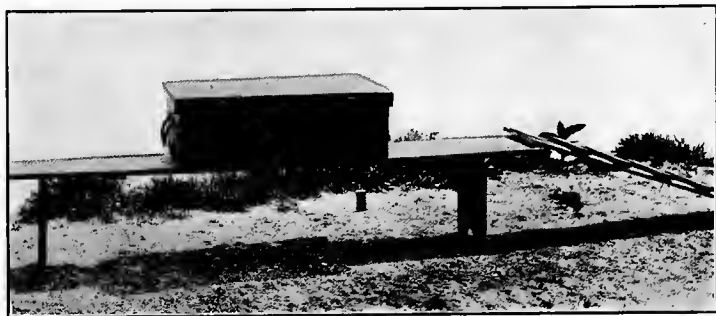
FIG. 50.—Makeshift test incline and fitting platform for use in the field composed of a sea box, mess bench and two planks.
