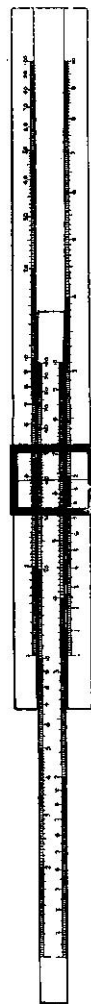
Fig. 34.—Setting for dividing 197 by 6.35. Hair-line of cursor on 1.97 on D. 6.35 on C set under hair-line.
