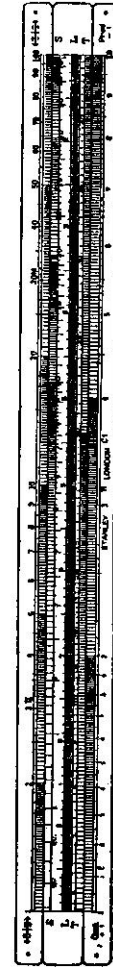
Fig. 4.—The slide reversed for sine and tangent calculations. The sine is read off on A over the given angle on S.
