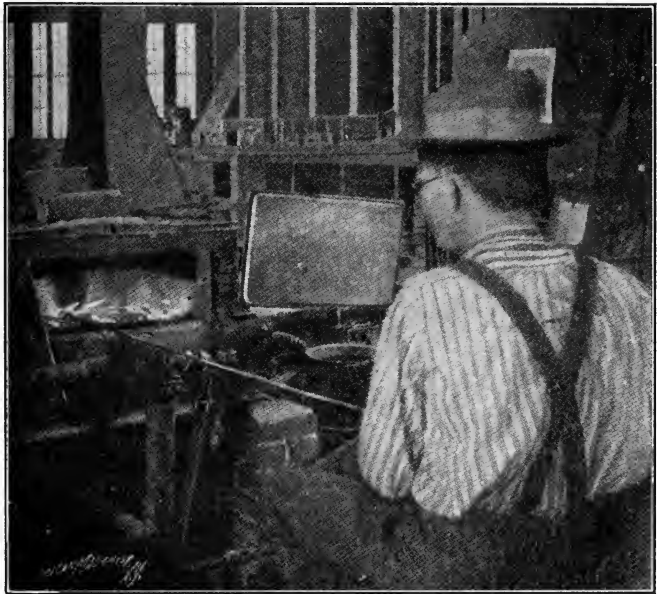
FIG. 205.—Heating flanges in muffle, using natural gas.
