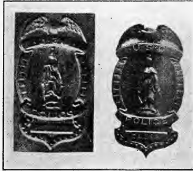
FIG. 79.—Embossed Police-shield before and after trimming.
