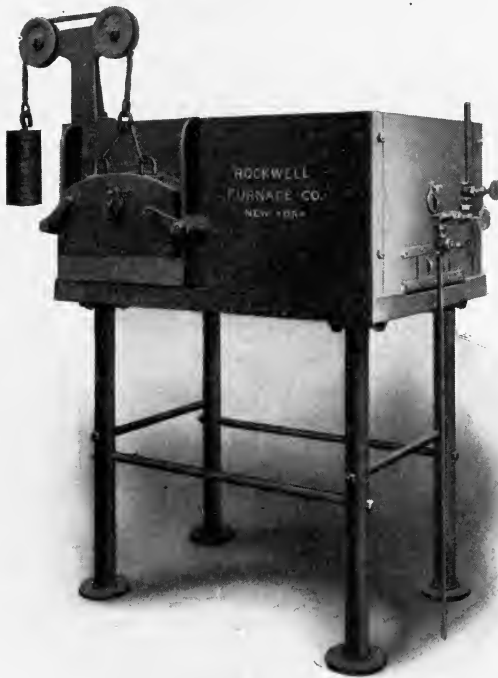
FIG. 163.—End-heating forge furnace.
