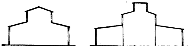
Fig. 100.—Simple Forms of Monitor-Light Roof Constructions
