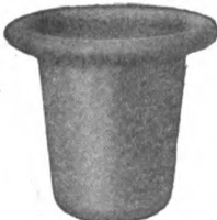
Fig. 204. Cast-Iron Pot Used for Lead Pot
