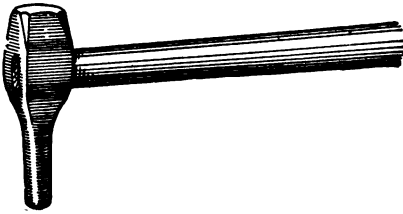
Fig. 51. Punch for Heavy and Fast Work
