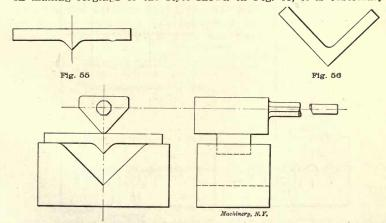
Fig. 57 Figs. 55 to 57. Forging an Angle Iron
