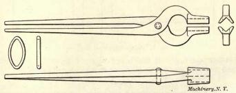
Fig. 9. Tongs with V-shaped Jaws
