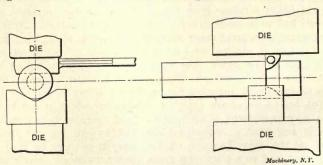
Fig. 49. Use of Breaking-down Tool and V-block in the Steam Hammer
