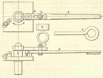
Fig. 19. Tool for Forging Open Eye-bolts or Hooks
