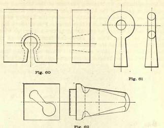
Figs. 60 to 62. Trimming Die and Punch and Completed Work
