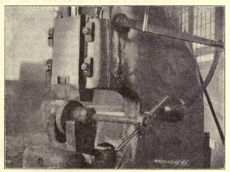
Fig. 66. Steam Hammer Fixtures used when Forging Rings
