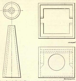
Fig. 15. Taper Cone for Forging Rings, Collars, etc.
