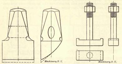
Fig. 5. Correct and Incorrect Shape of Blacksmith's Breaking-down Tool
