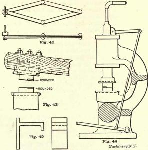
Fig. 42. Gage for Setting Adjustable Die to Any Angle. Fig. 43. Common, but Objectionable, Way of Placing Dies in Helve Hammer. Fig. 44. General Appearance of Pneumatic Hammer for Light Forging. Fig. 45. Piece that can be forged to Advantage in the Forging Machine
