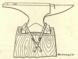
Fig. 25. Objectionable Manner of Holding an Anvil in Position
