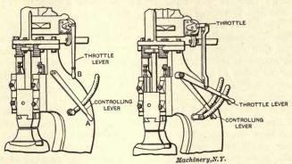
Fig. 33. Single Frame Steam Hammer, showing Common Arrangement of Levers
