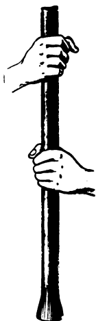
Fig. 84.—Jumping Bar Vertically.
