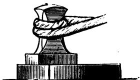
Fig. 89.—Smoothing Faces of Ring with Flatter.
